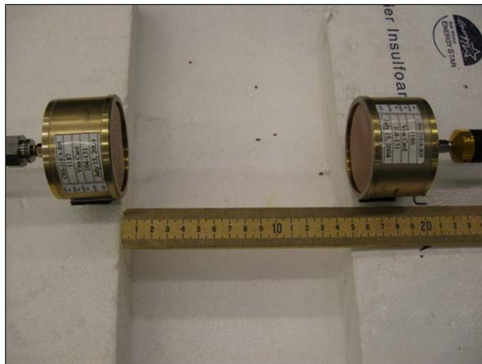
Figure 2 Image of the antennas used for the 2 GHz to 10 GHz band
