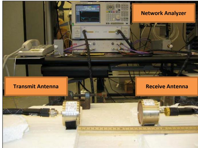
Figure 1 Image of Network Analyzer and the 2 GHz to 10 GHz band antennas
