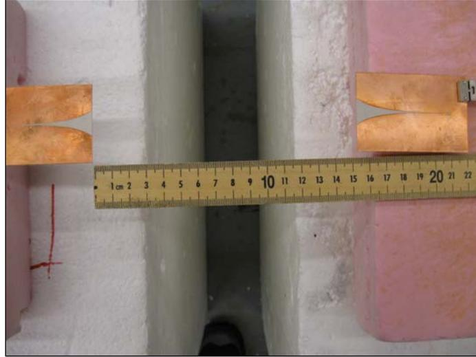
**Figure 3** Image of the antennas used for the 10 GHz to 40 GHz band
